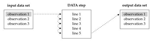
This diagram illustrates how an observation flows through a DATA step:
